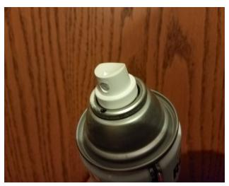
The dot on a spray can is used to show the position of the pickup tube in the bottom of the can. Position the nozzle toward the dot if spraying downward. If tilting the can upward, position the nozzle away from the dot.
