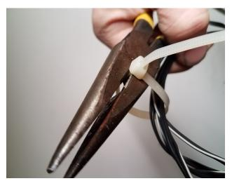
Tie wraps can be re-used if cut properly. Just cut it on the side shown and pull the cut end through. You now have a reusable tie wrap (for a smaller bundle)
